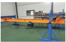
Suspension end carriage drive by gear motor, advocate material by hot-rolled steel, bridge on the tooth and bilateral wheel driving, simple structure, light weight, space utilization rate is high, running smooth and noise low. It's good partner of suspension crane manufacturing.
