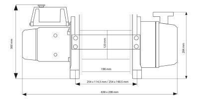
Rope Diameter / Diámetro del Cable: 7 / 13 in | 13.8 mm Drum Size: Ø 4.72" x 7.8" | Ø 120 mm x 198 mm
