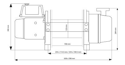
Rope Diameter / Diámetro del Cable: 7 / 13 in | 13.8 mm Drum Size: Ø 4.72" x 7.8" | Ø 120 mm x 198 mm
